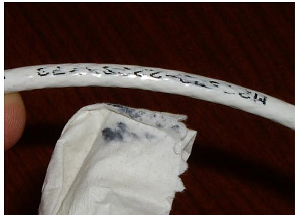
Marking with an ink jet system is also prone to fade in the long run. While liquids can immediately compromise the wire identification mark, time can also cause the ink to fade, which is especially a concern in the harsh environment of an aircraft. This leads once more to perfectly good wire being discarded, increasing supply costs and using up resources. LASELEC's laser identification is permanent; as long as the wire exists, so will the marking.
